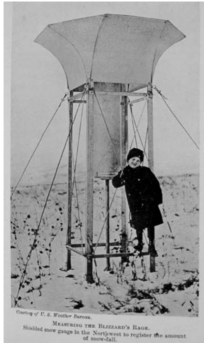
Figure 4.1 Shielded snow gauge in the northwest United States used to register snow fall (courtesy National Oceanic and Atmospheric Administration (NOAA), NOAA Central Library, NOAA Photo Library, wea 00901, Historic NWS Collection, original photo, US Weather Bureau, 1917 in “Boy with Weather Men,” p. 224)
