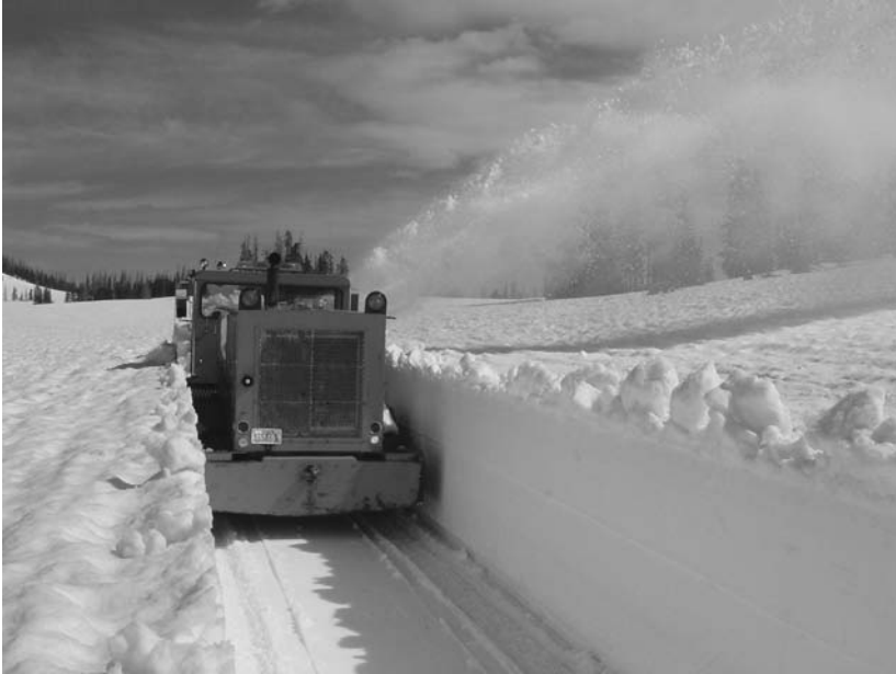
Figure 1.5 Transportation department snow blower at work clearing Highway 143 between Cedar Breaks and Panguitch, Utah in 2005. (Courtesy R. Julander.) See also color plate.
