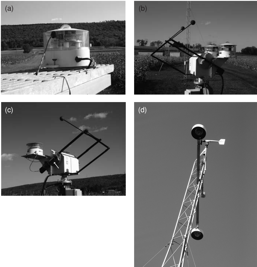
Figure 6.1 Radiation instruments at the Penn State, Pennsylvania SURFRAD Network site: (a) pyranometer used to measure incoming shortwave radiation on a horizontal surface, (b) a continuously shaded pyranometer (near) and pyrgeometer (far) used to measure incoming diffuse shortwave and incoming longwave radiation, respectively, (c) tubular pyrheliometer (see arrow) mounted on a solar tracker to measure direct-beam solar radiation at normal incidence, and (d) inverted pyranometer and pyrgeometer on tower to measure reflected shortwave and outgoing longwave radiation from the ground surface (photographs by D. DeWalle). See also color plate.
