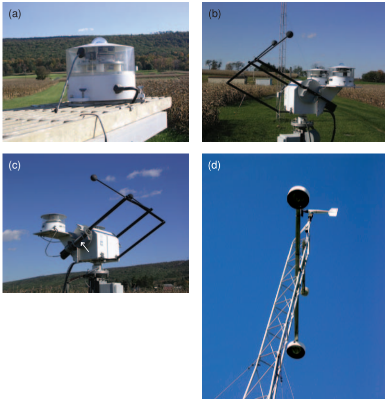
Figure 6.1 Radiation instruments at the Penn State, Pennsylvania SURFRAD Network site: (a) pyranometer used to measure incoming shortwave radiation on a horizontal surface, (b) a continuously shaded pyranometer (near) and pyrgeometer (far) used to measure incoming diffuse shortwave and incoming longwave radiation, respectively, (c) tubular pyrliometer (see arrow) mounted on a solar tracker to measure direct-beam solar radiation at normal incidence, and (d) inverted pyranometer and pyrgeometer on tower to measure reflected shortwave and outgoing longwave radiation from the ground surface (photographs by D. DeWalle).
