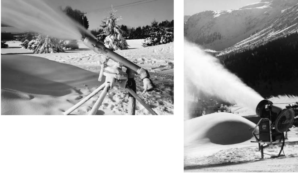
Figure 12.11 Ratnik low-energy modified snow gun (left) and modified fan-type Lenko snow gun (right) being used to augment snowpack for skiing (courtesy of Ratnik Industries, Inc. and Lenko Quality Snow, Inc., respectively). See also color plate.
